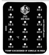
The P8003 Irreversible Temperature Indicator is a threshold temperature indicator with 16 temperature intervals (ranging from 27.5°C to 65.0°C), and a stated accuracy of ±1°C for each temperature interval event. Color development is activated at each temperature interval event, and the color development displays on the label window specifying the temperature event. The color changes from white to red, and the red color is irreversible and will not revert to the original state of white.
